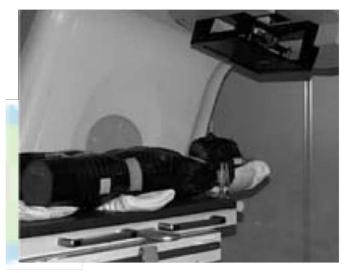
**Figure 4.** An adult female RANDO phantom on the LINAC table to measure the exposure doses to the inner pelvis after irradiation of the simulated cerebral AVM with 20Gy.
