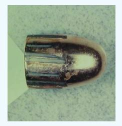
Figure 2: Recovered bullet with rifling marks important forensic evidence that can easily be damaged without proper surgical precautions.
