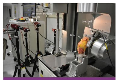
**Figure 3.** Test set-up for biomechanical evaluation of the joint using the robotic testing system (Technology Service Ltd., Model FRS2010, Chino, Japan). An optical tracking system was used to assess strain in the lateral capsule during different loading conditions.
