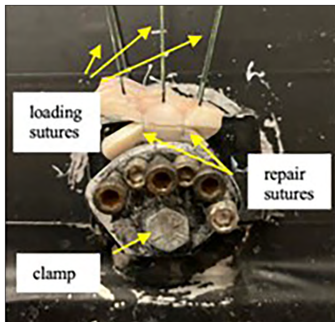
Figure 1. Clamped inner edge of meniscus wedge with three loading sutures placed at the peripheral rim
