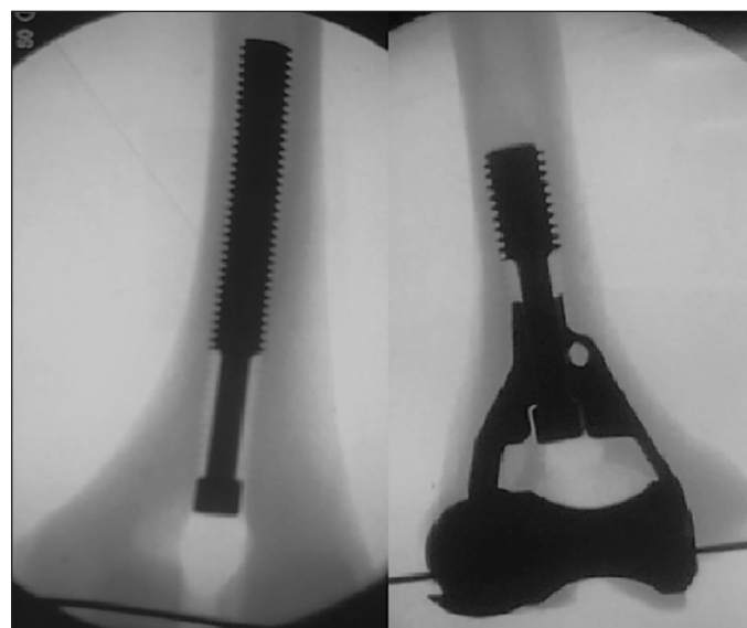
Figure 2. Screw insertion into 3D-printed models. Radiograph of test construct pictured left. Implant body is included (overlapped) for reference, pictured right.
