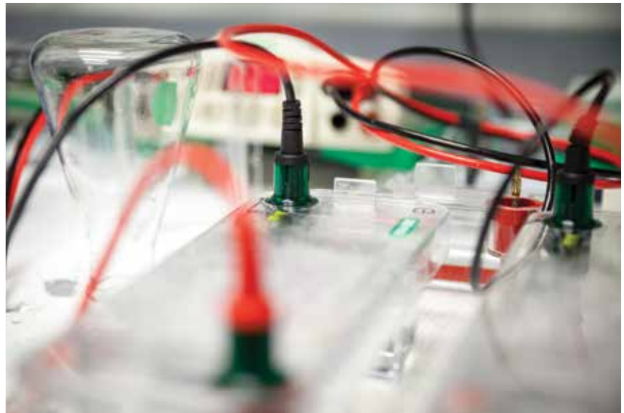
Detail of gel electrophoresis device inside the Charles and Louella Snyder Laboratory for Retinal Regeneration.
