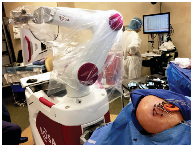
Figure 1: The ROSA robotic arm in the “home” position, after placement of several right temporal depth electrodes during a recent SEEG case. Julie Pan, MD, PhD, an epilepsy neurologist, evaluates the intracranial recordings in the background.
