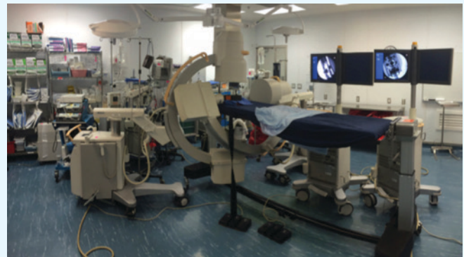
Figure 2. Two Philips C-arm fluoroscopes positioned perpendicularly to each other near a radiolucent Jackson table to simulate the workflow for interventional cases. Note the lateral fluoroscopic arm canted toward the foot of the bed in order to prevent the two machines from colliding. The displays show anteroposterior and lateral images taken simultaneously with overlapping regions of interest.
